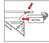
**Step 3** Remove the battery (See battery installation page)
