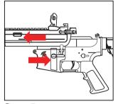
**Step 5** Slide the upper receiver away from the lower receiver.
