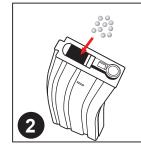
**Step 2** Pour BBs into the magazine. Do not overfill. Use high quality 0.20g or heavier BBs.\*
