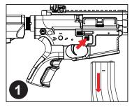
Step 1 Press the mag release button to remove magazine.
