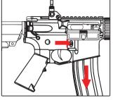
Step 1 Place the selector switch to safe & fully retract the stock.
