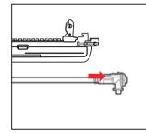
**Step 6** Slide the inner barrel and hop-up assembly out of the upper receiver.
