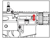
Step 3 Turning the dial downward will cause the BB to float upwards, whereas turning the dial upward causes the BB to fall downward.
