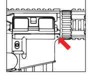
Step 8 Align the front pin with the lower receiver. Push in the pin to secure both receivers.
