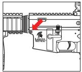
**Step 4** Unscrew front pin with hex key. Tap the front body pin out until the upper receiver disconnects.
