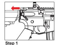
Pull the charging handle back to move the bolt plate back, thus exposing the hop-up adjustment dial. Hold in place while adjusting the hop-up.
